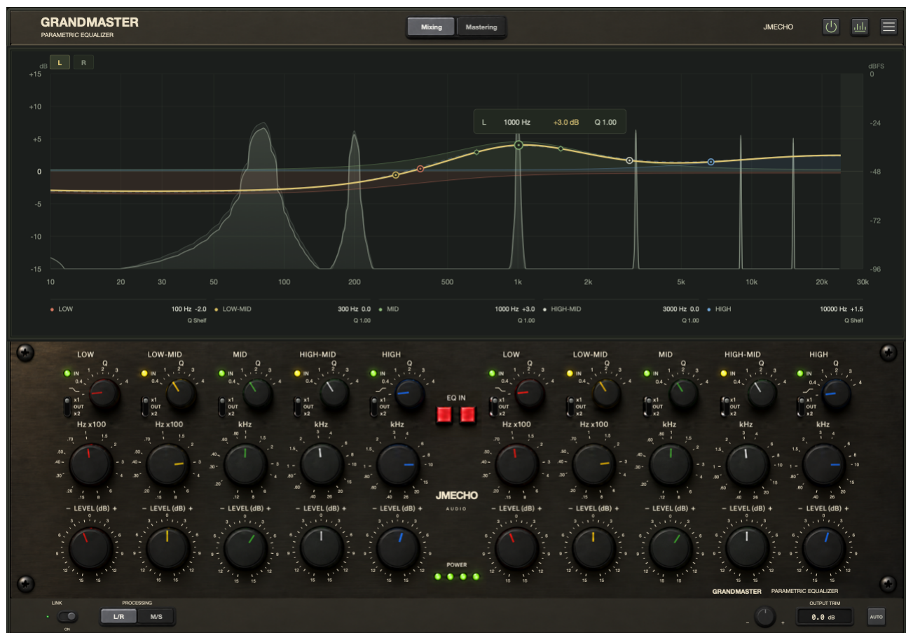
Figure 8. Native capture using generated six-tone test PCM: 96 kHz processing and 48 kHz FFT analysis. Input tones are 80, 200, 1000, 3200, 9000 and 15000 Hz. Mixing EQ settings are a 100 Hz low shelf at -2 dB, a 1 kHz Bell at +3 dB / Q 1 and a 10 kHz high shelf at +1.5 dB. Trim is 0 dB; AUTO, ADDA and noise are off.
