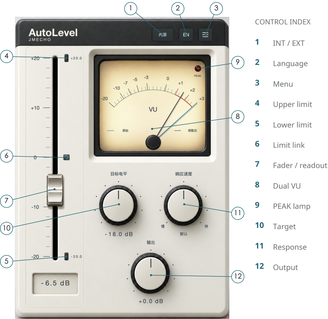
Figure 1. The actual AutoLevel 0.10.9 Chinese panel and control index. Controls correspond across both languages. Displayed playback values are examples rather than defaults.
