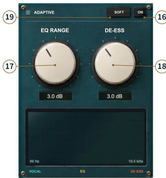
Figure 6. ADAPTIVE controls 16-19. The dB values set processing ranges or limits, not a constant reduction.
