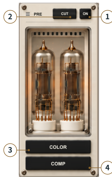
Figure 2. PRE controls 1-4. LOW CUT precedes preamp coloration and compression; switches are enabled in this view.
