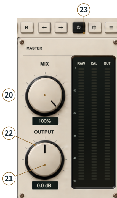
Figure 7. MASTER controls 20-23. Entry 22 points to the OUTPUT hover area for AUTO; the button appears on hover or during measurement. Global power, 23, is in the top bar.
